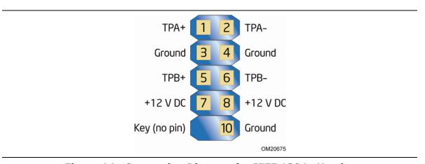
Figure 14. Connection Diagram for IEEE 1394a Header
